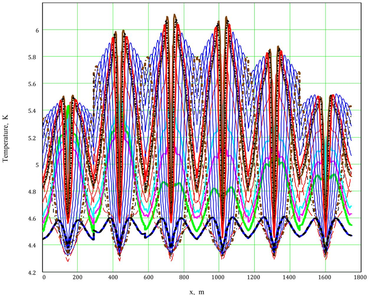
**Figure 6.** Variation of CICC temperature in 6 middle double pancakes of six CS sections CS3L, CS2L, CS1L, CS1U, CS2U, CS3U during a 1800 s plasma pulse. Normal operation
