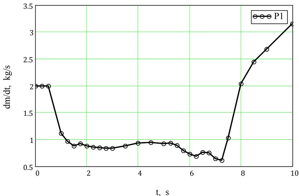
*Flow rate variation of circulator P1 in accordance with its characteristic  $\dot{m} - \Delta P$*
