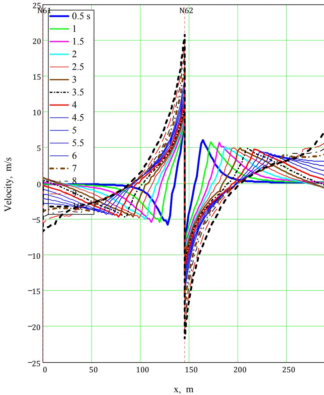
*Helium velocity in cable space for adjacent pancakes #61 and #62 of quenched CS section CS2L*
