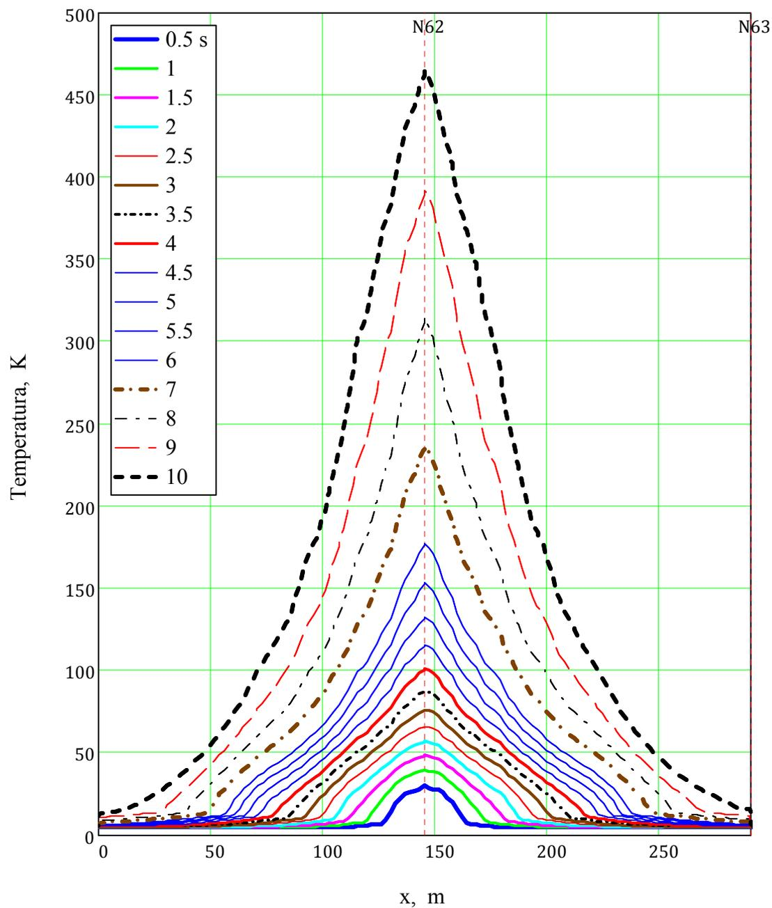
*Temperature evolution of CICC bundle for adjacent pancakes #61 and #62 of quenched CS section CS2L*
