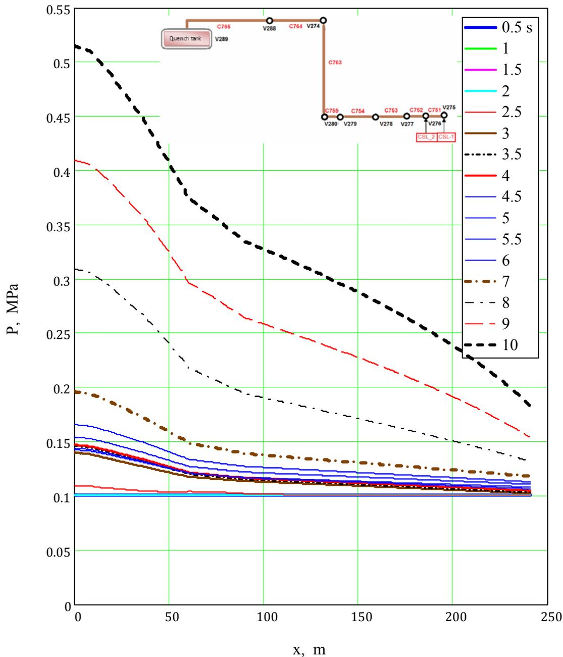
*Evolution of pressure along selected portion of quench lines (see total layout of quench lines in Fig. 5)*
