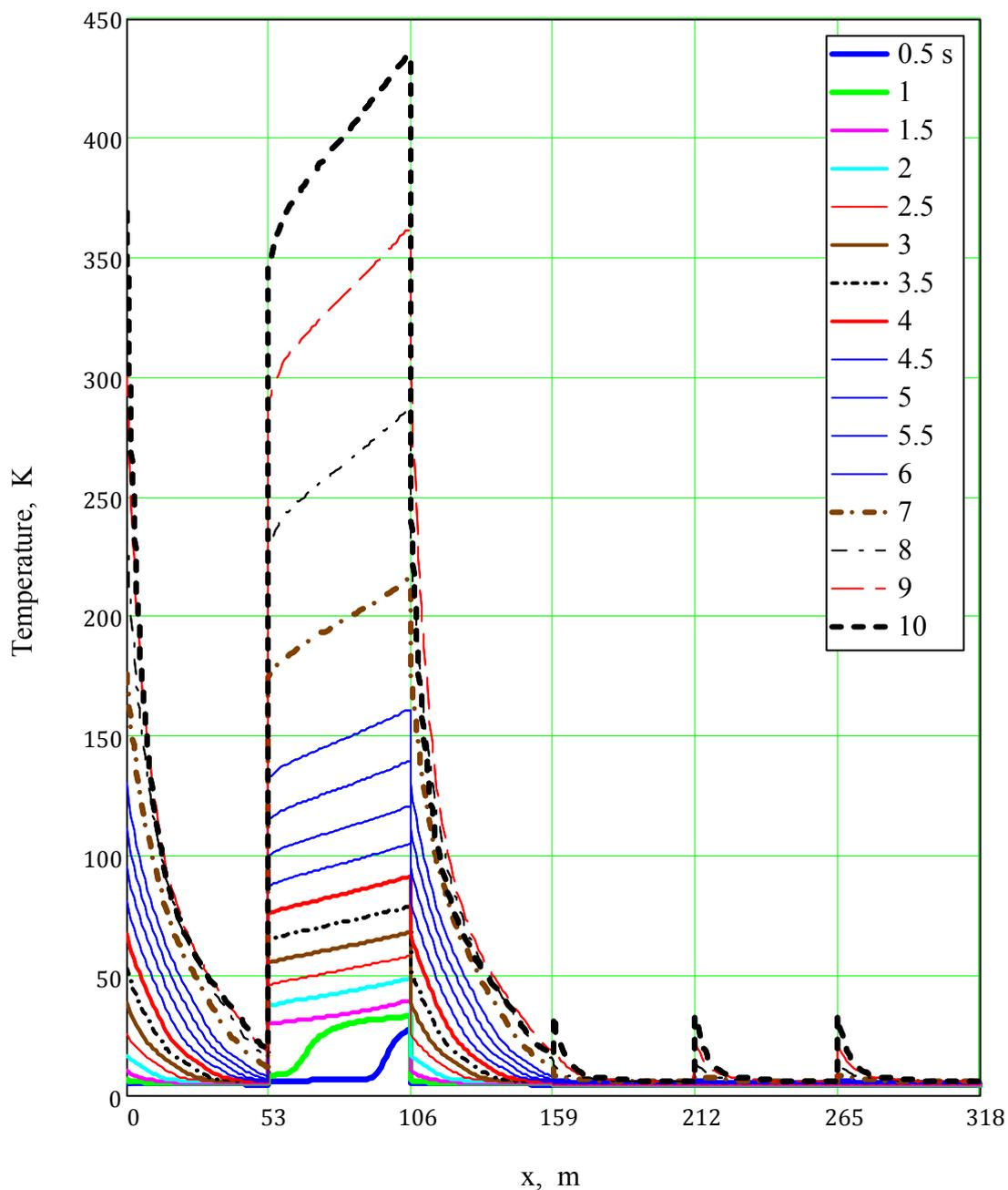
*Helium temperature variation in 6 inlet feeders (C733, C734, C735, C736, C737, C738, each 53 m in length) for six CS sections: CS3L, CS2L, CS1L, CS1U, CS2U, CS3U*
