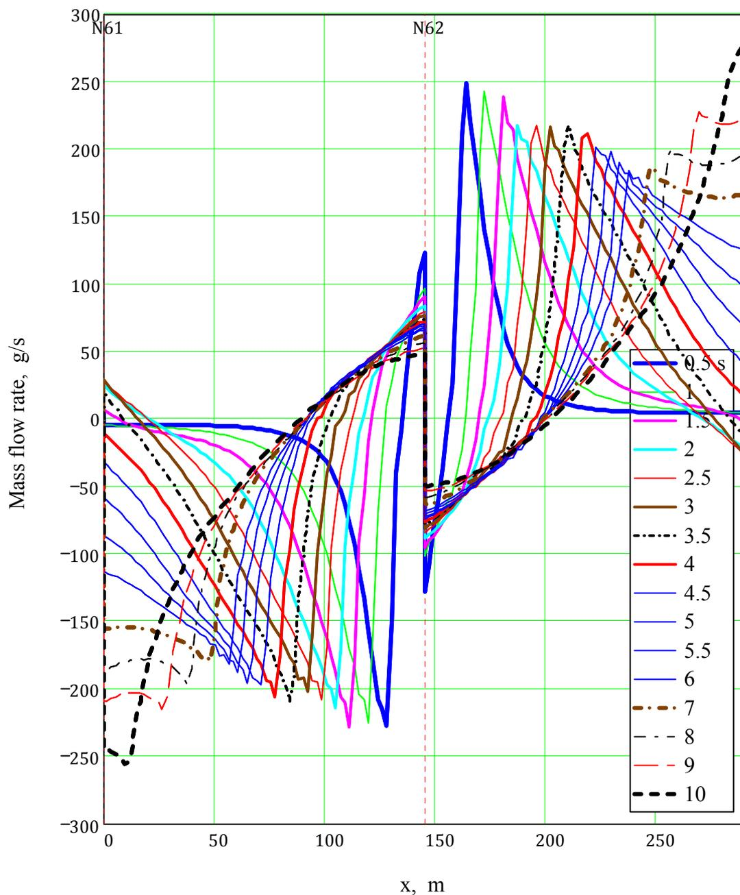
*Helium mass flow rate in cable space for adjacent pancakes #61 and #62 of quenched CS section CS2L*
