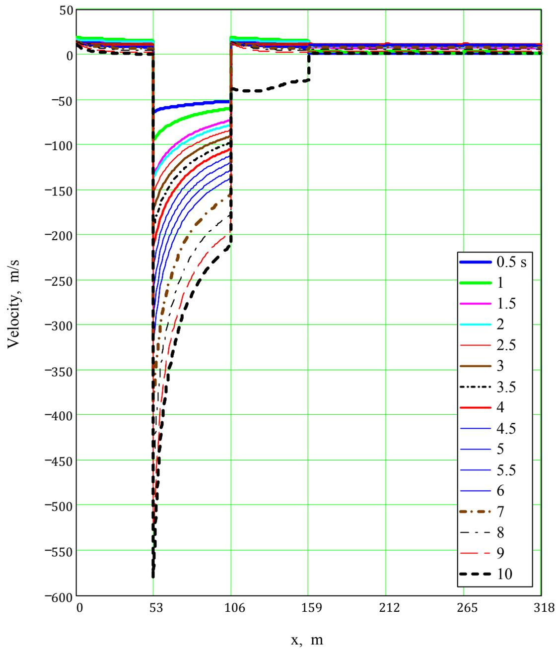
*Helium velocity variation in 6 inlet feeders for six CS sections*
