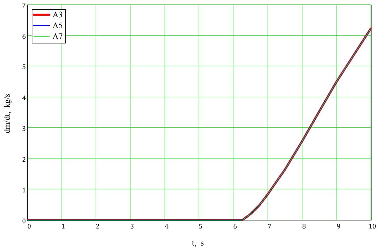
*Helium mass flow rate at inlets of relief valves A3, A5, A7*
