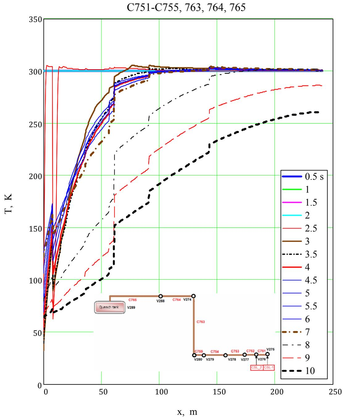
*Evolution of temperature along selected portion of quench lines (see total layout of quench lines in Fig. 5)*
