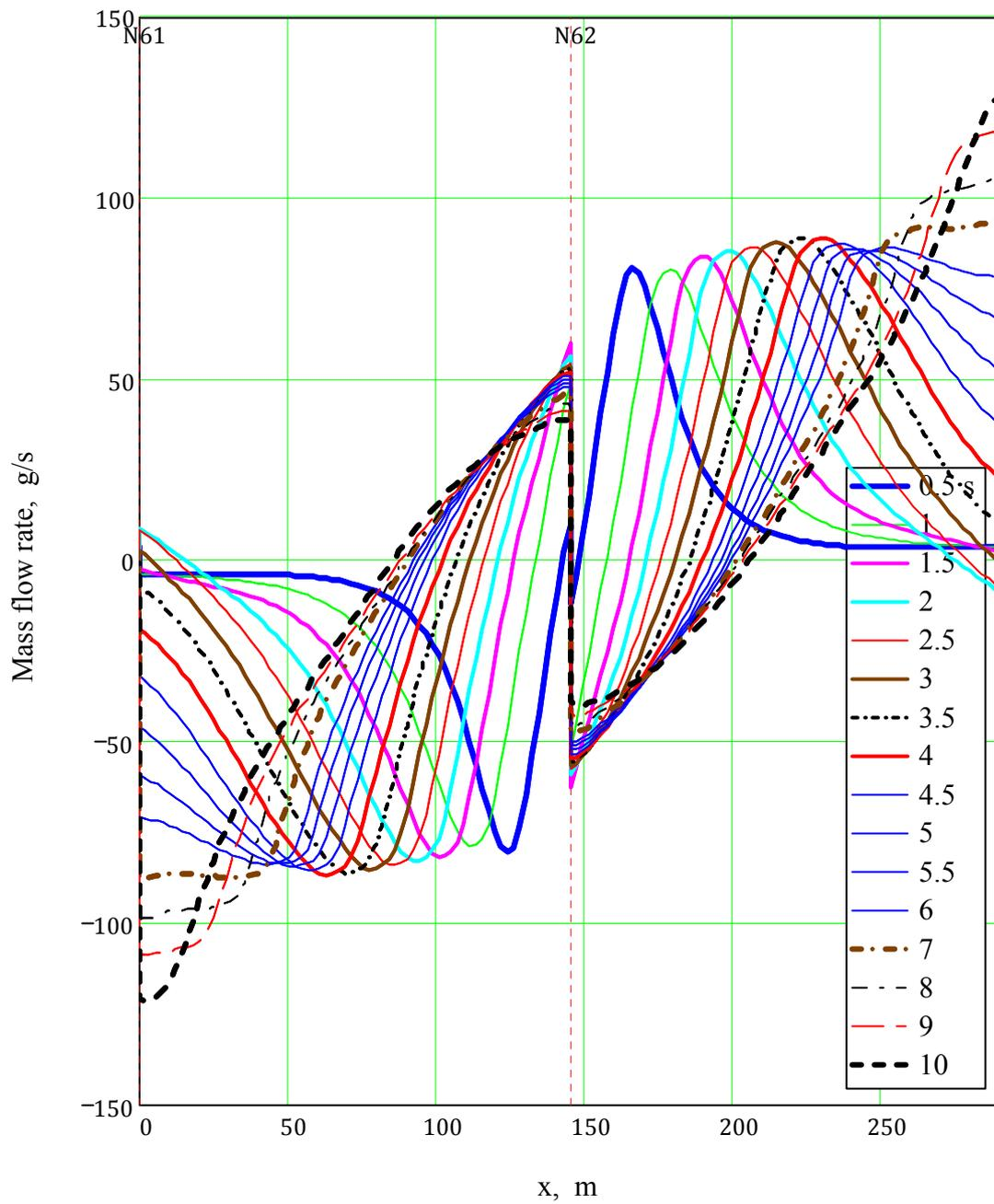
*Helium mass flow rate in central channel for adjacent pancakes #61 and #62 of quenched CS section CS2L*
