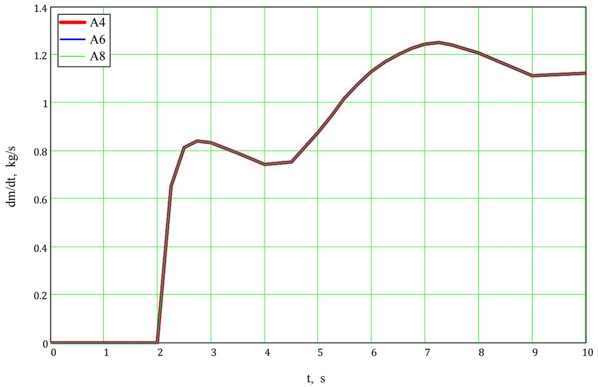
*Helium mass flow rate at inlets of relief valves A4, A6, A8*
