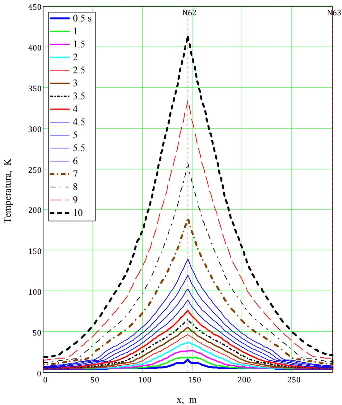
*Helium temperature evolution in central channel for adjacent pancakes #61 and #62 of quenched CS section CS2L*
