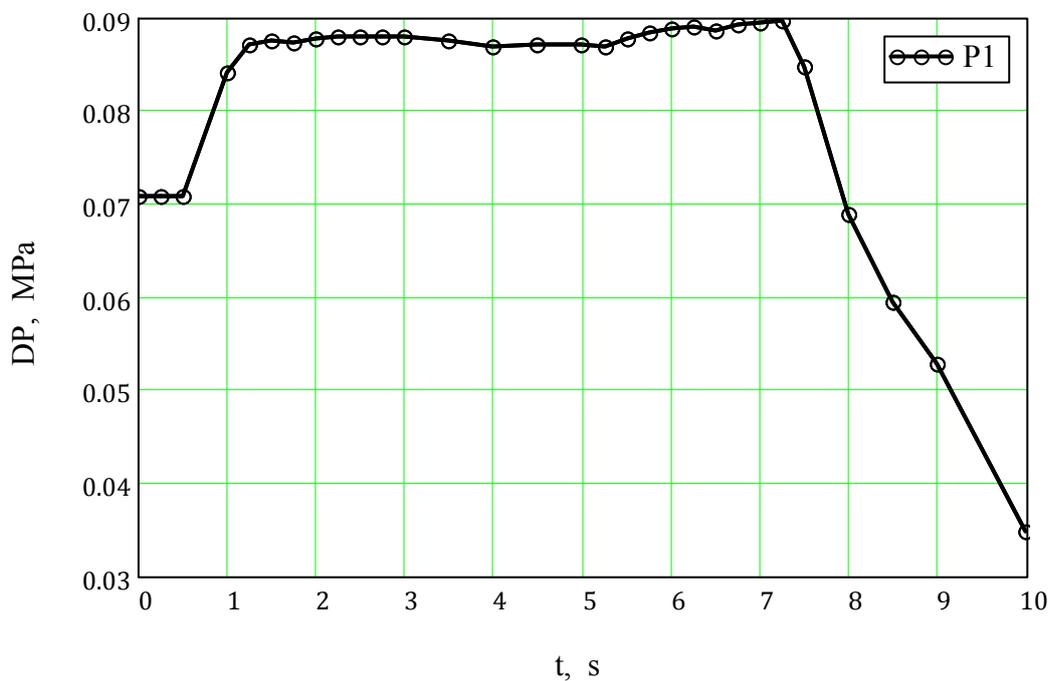
*Pressure head variation in circulator P1 limited by control valve A2 opening*
