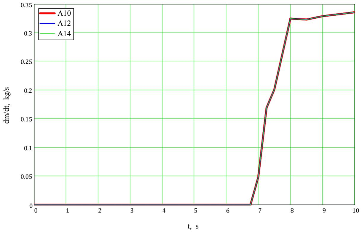
*Helium mass flow rate at inlets of relief valves A10, A12, A14*
