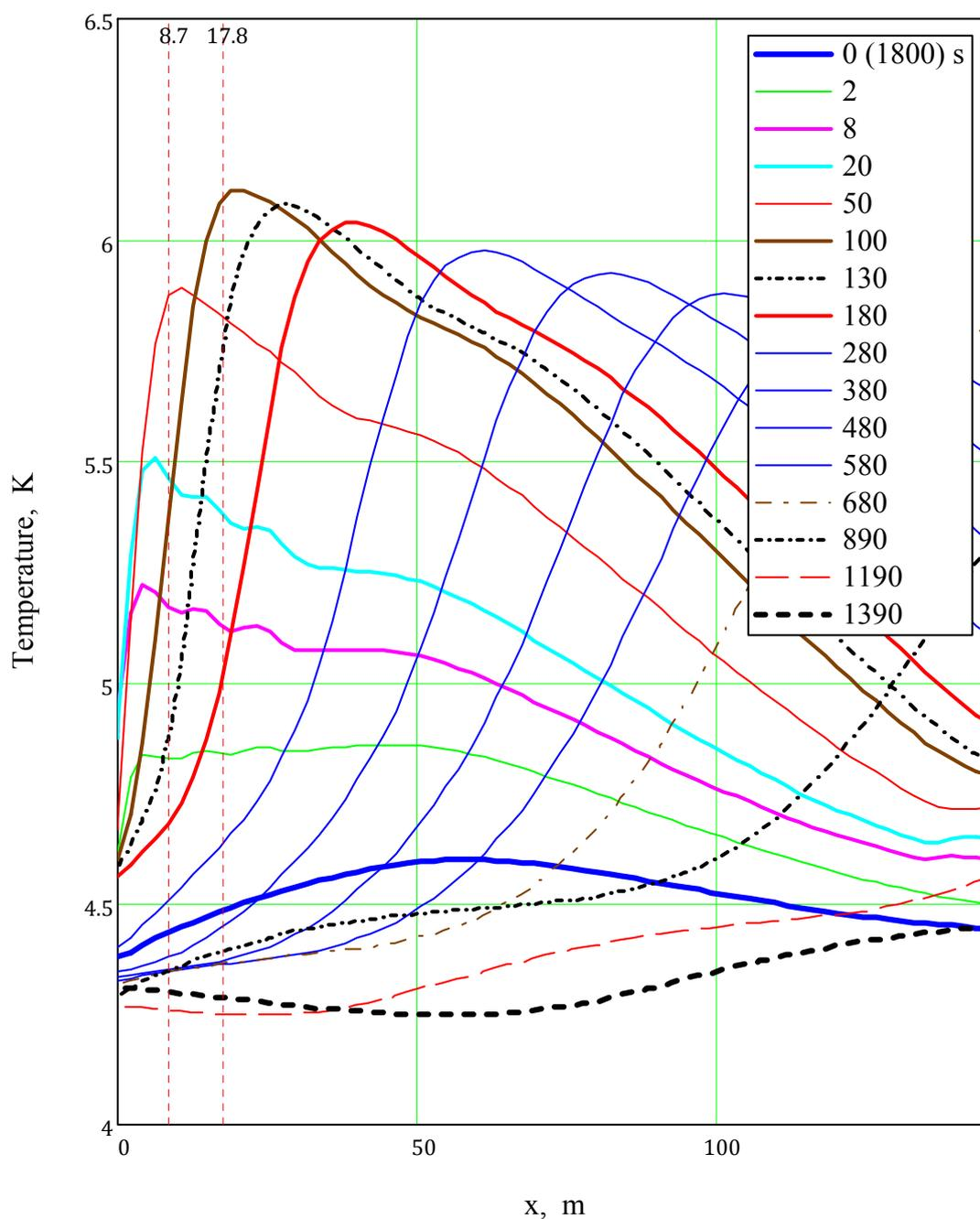
*Figure 7. Temperature variation along pancake #102 (middle of CS1L). Normal operation*
