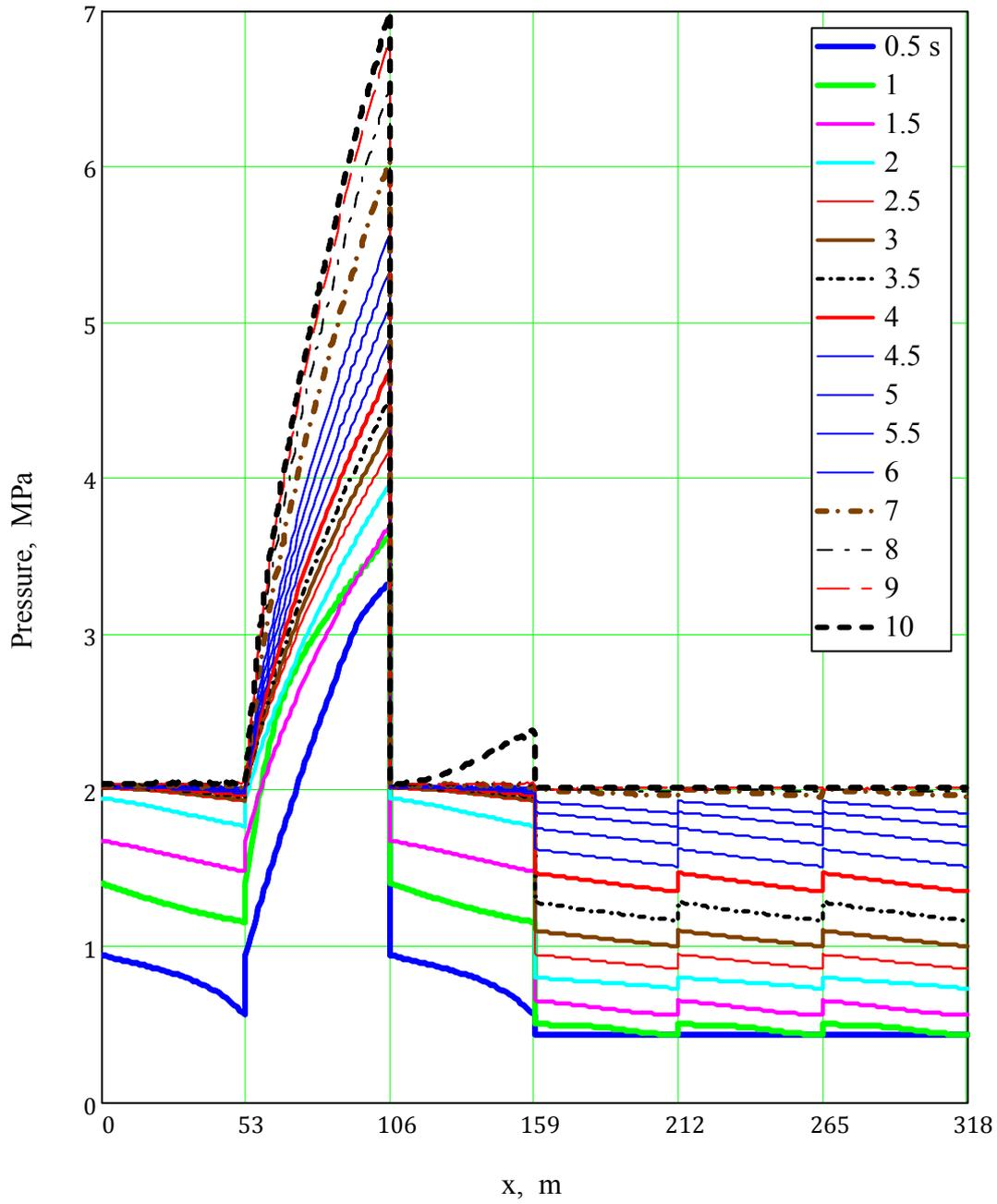
*Helium pressure variation in 6 inlet feeders for six CS sections*
