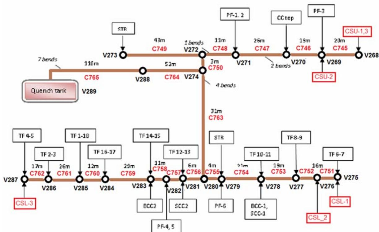
Figure 5. Hydraulic scheme of quench lines
