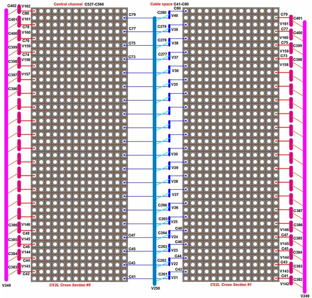
Figure 4. Extraction from CS hydraulic model: CS2L cooling circuit with position for cross sections #1 and #5
