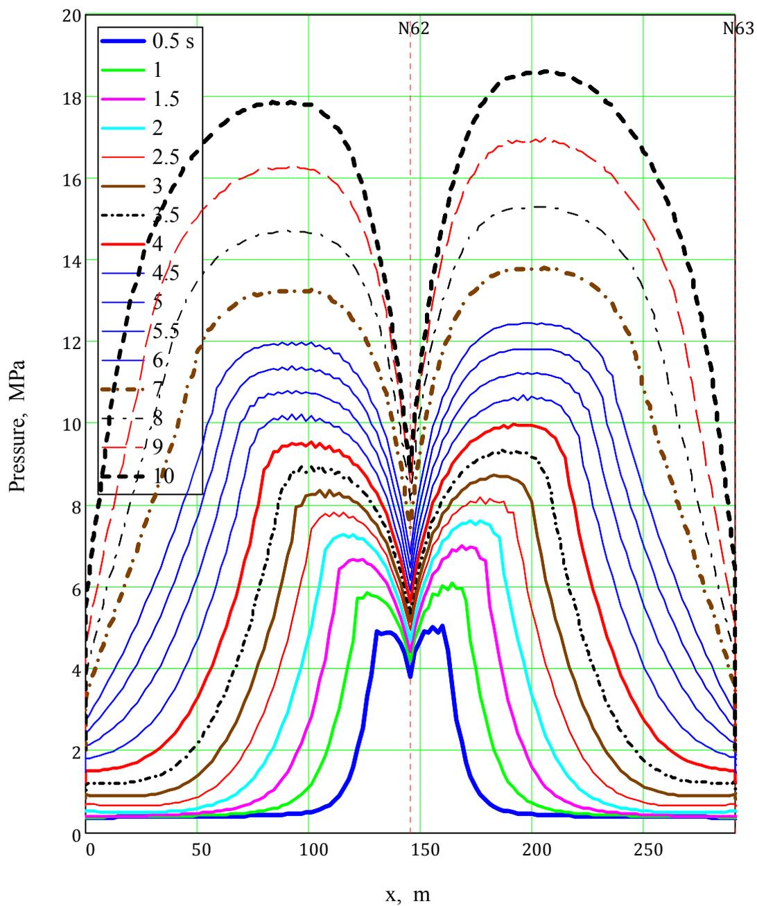
*Helium pressure in cable space for adjacent pancakes #61 and #62 of quenched CS section CS2L*
