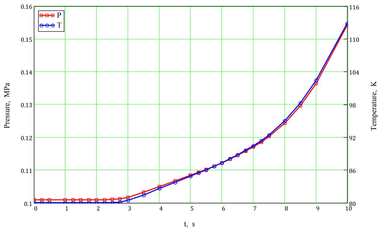
*Evolution of helium pressure and temperature inside quench tank V289 due to helium release via safety valves*
