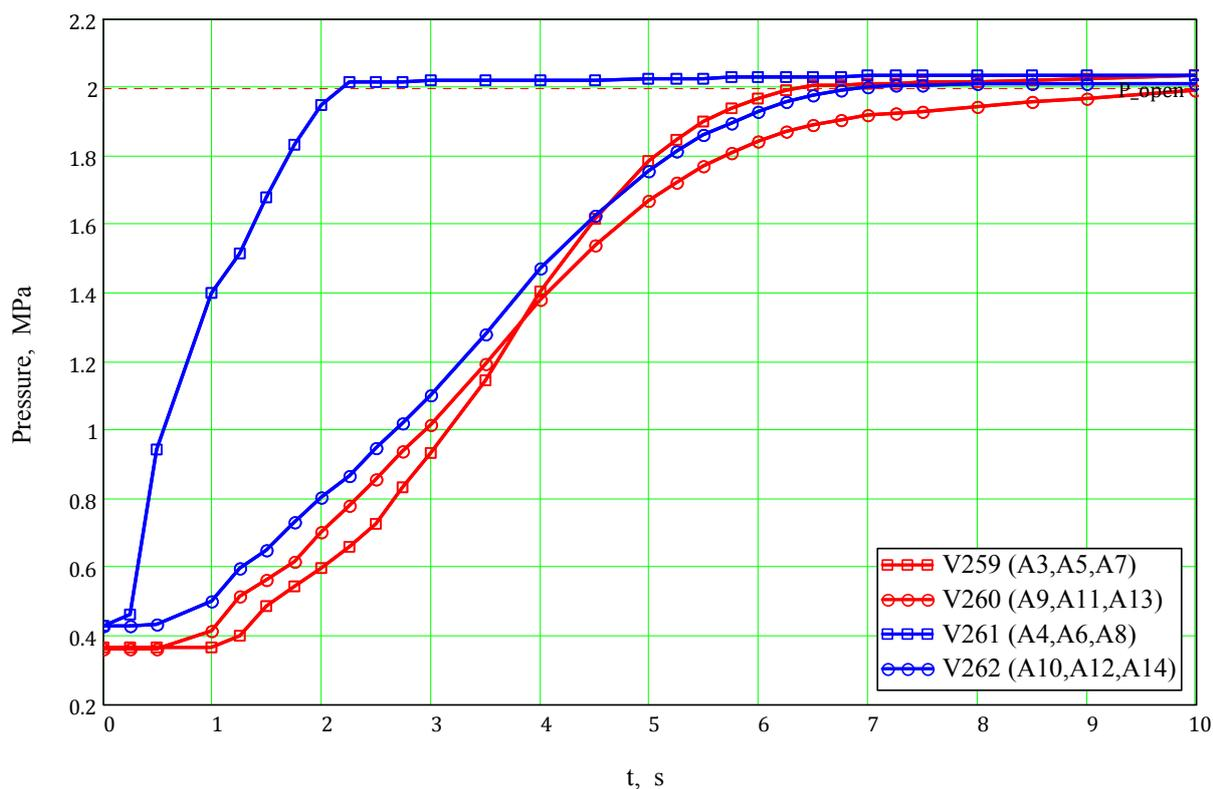
*Helium pressure at inlets of the safety relief valves*
