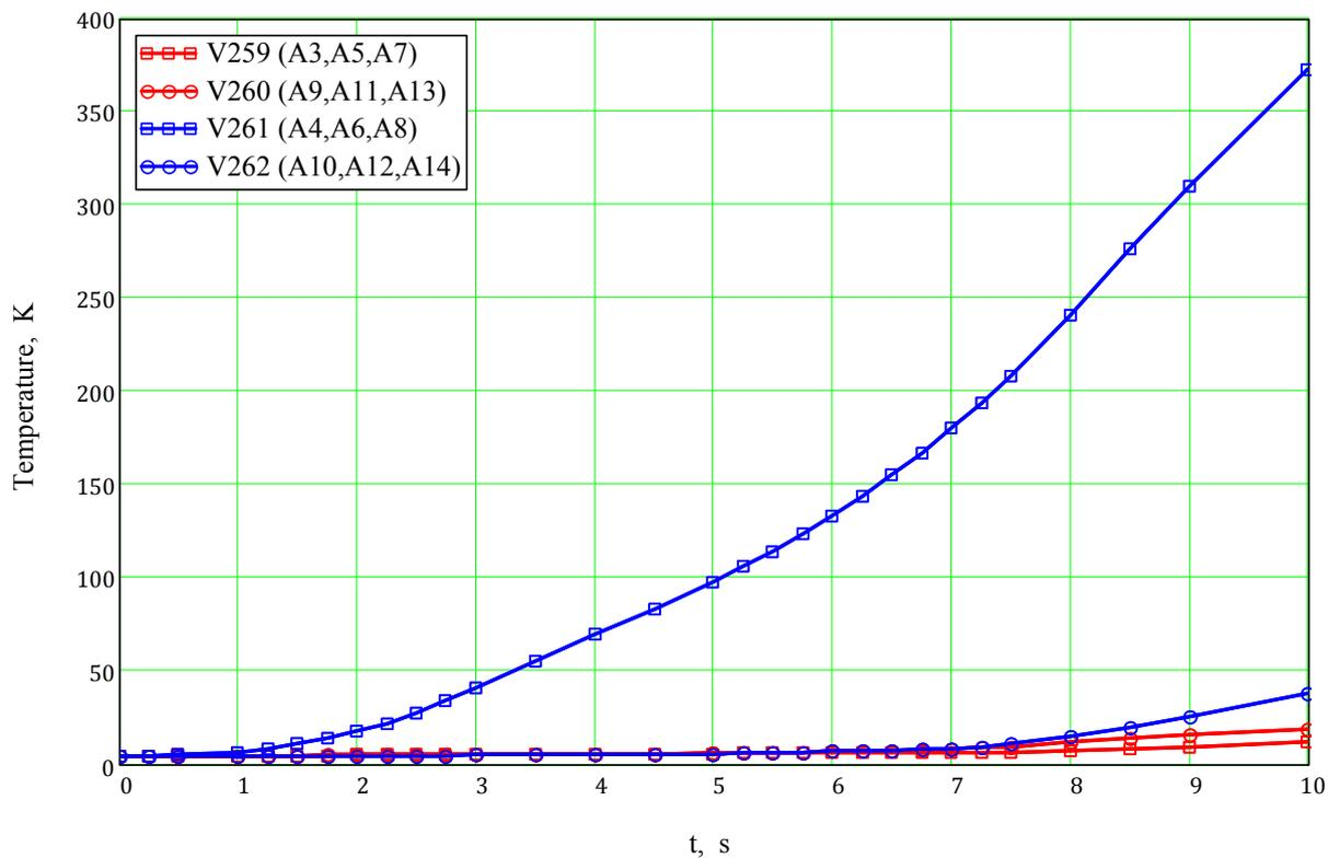
*Helium temperature at inlets of the safety relief valves*
