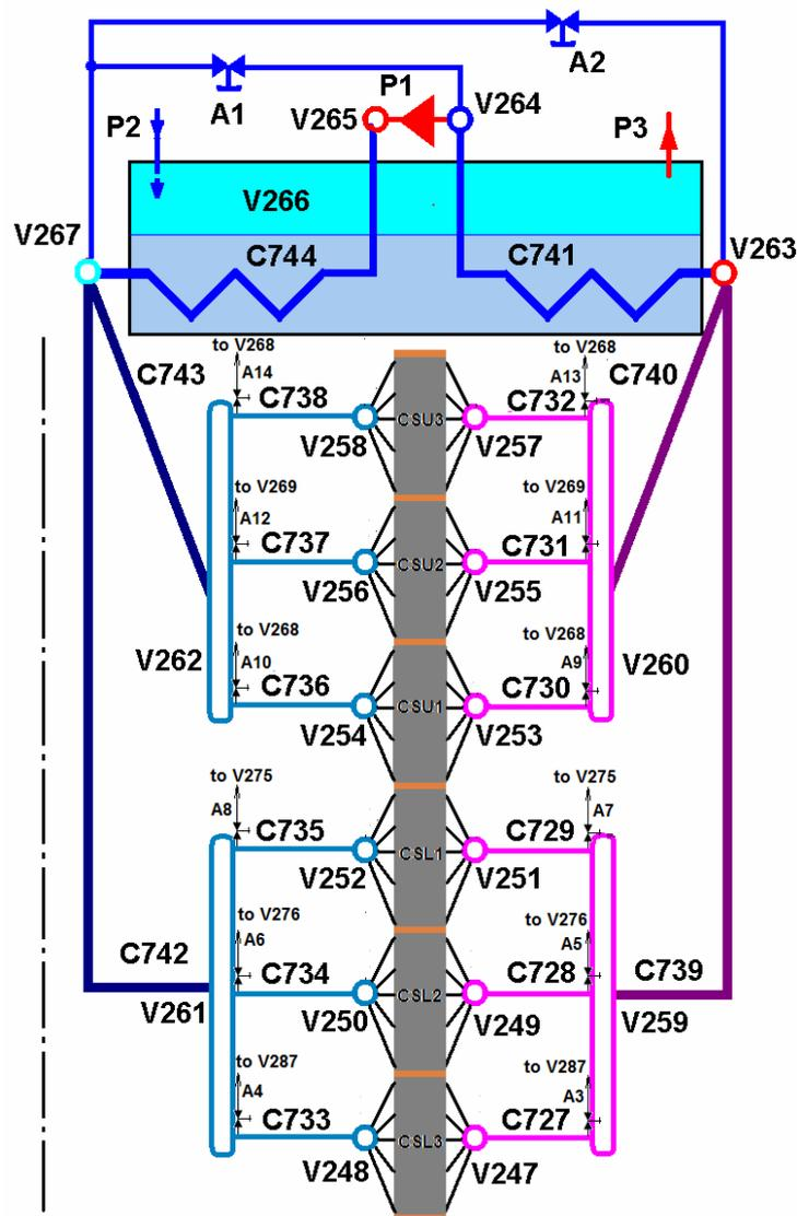
*Figure 2. Hydraulic scheme of CS cooling circuit.*
