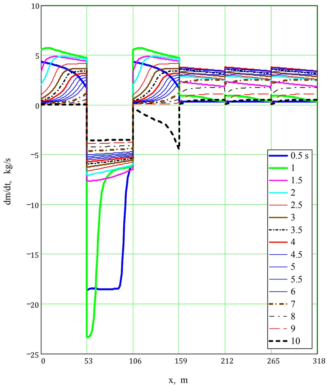
*Helium mass flow rate variation in 6 inlet feeders for six CS sections*
